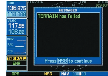
Figure 3-5: 'TERRAIN has failed' message
